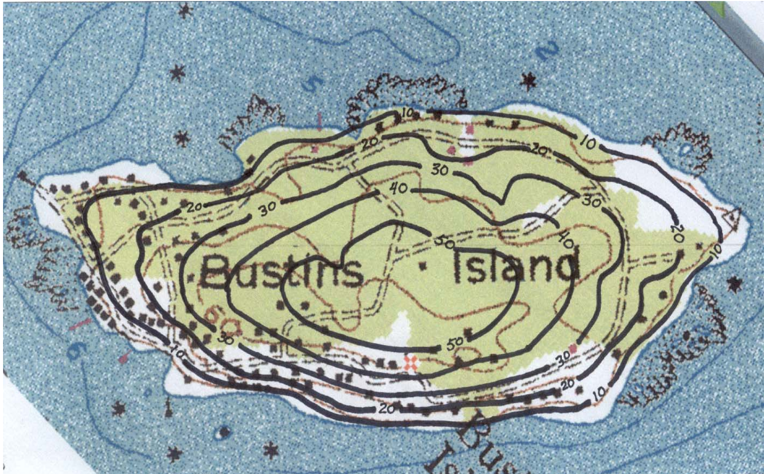
Figure 6: Head contours from the original RGGI steady-state model.
