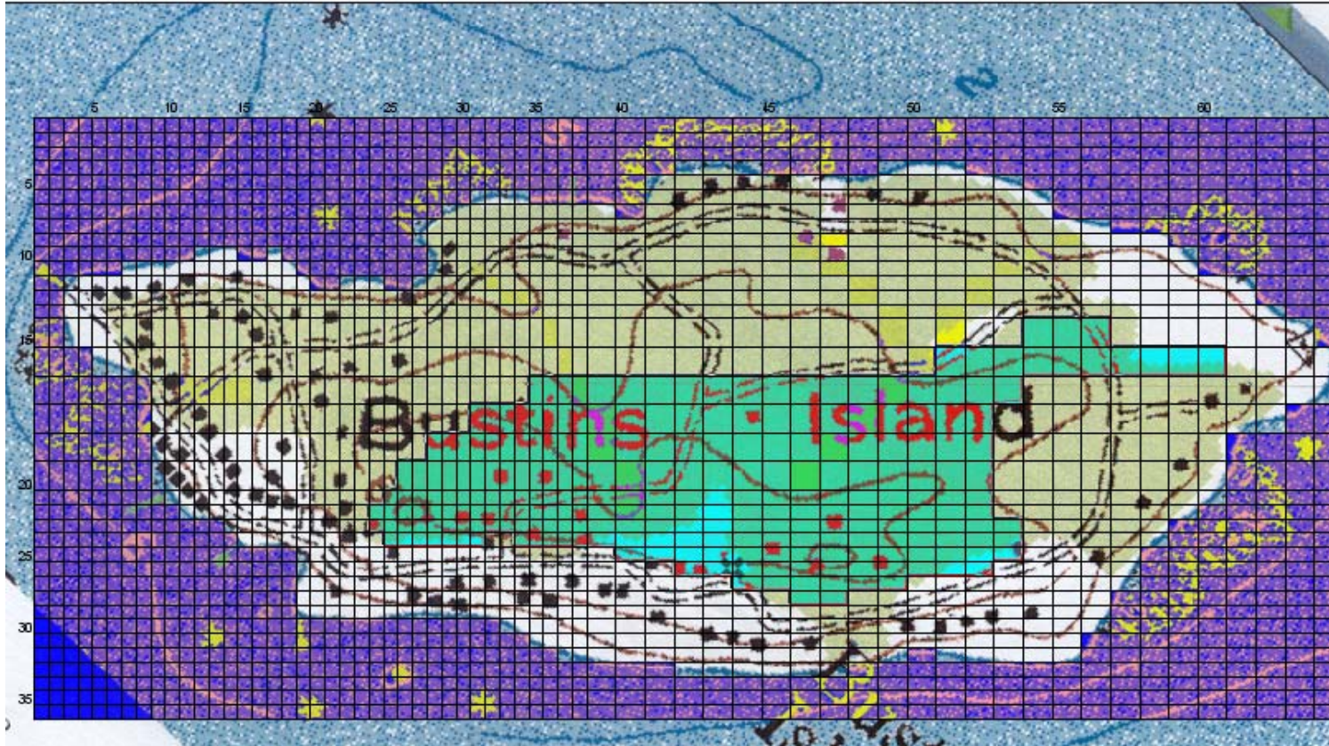
Figure 2: Zones of hydraulic conductivity for the bedrock. The green, low-K zone is surrounded by the higher K zone.
