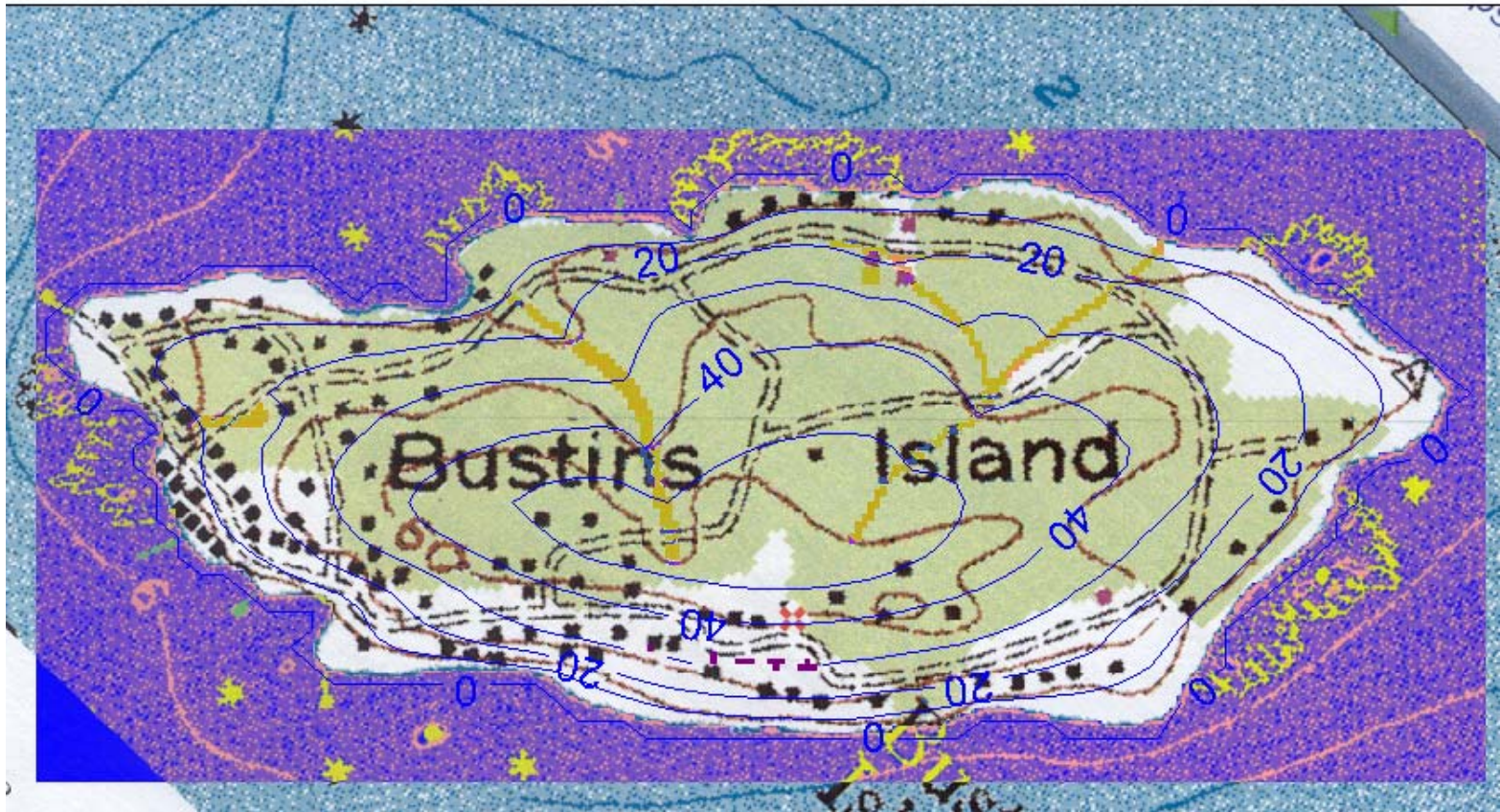
Figure 20. The model generated head contours for the refined model grid.
